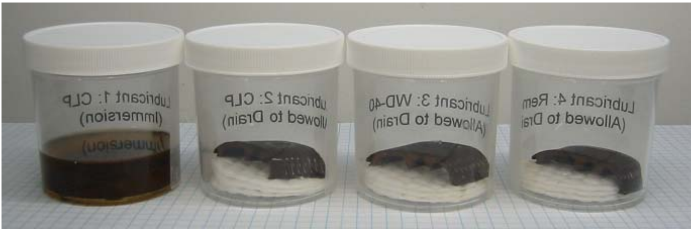
Figure 4 - Test pieces ready for storage
